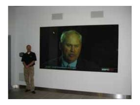
The large display is provided using only 9 feet of space behind the screen. This was accomplished with the use of a custom Da-Lite RPM Rear Projection Module. Up to 4 images can be displayed simultaneously through an Extron MGP-464 Quad Video Processor. A presentation is displayed in one of the quadrants, a slide show from an Extron GSS100 Graphic Still Store in another, and 2 DVD Movies using Pioneer professional DVD Players are shown in the last two quadrants.
