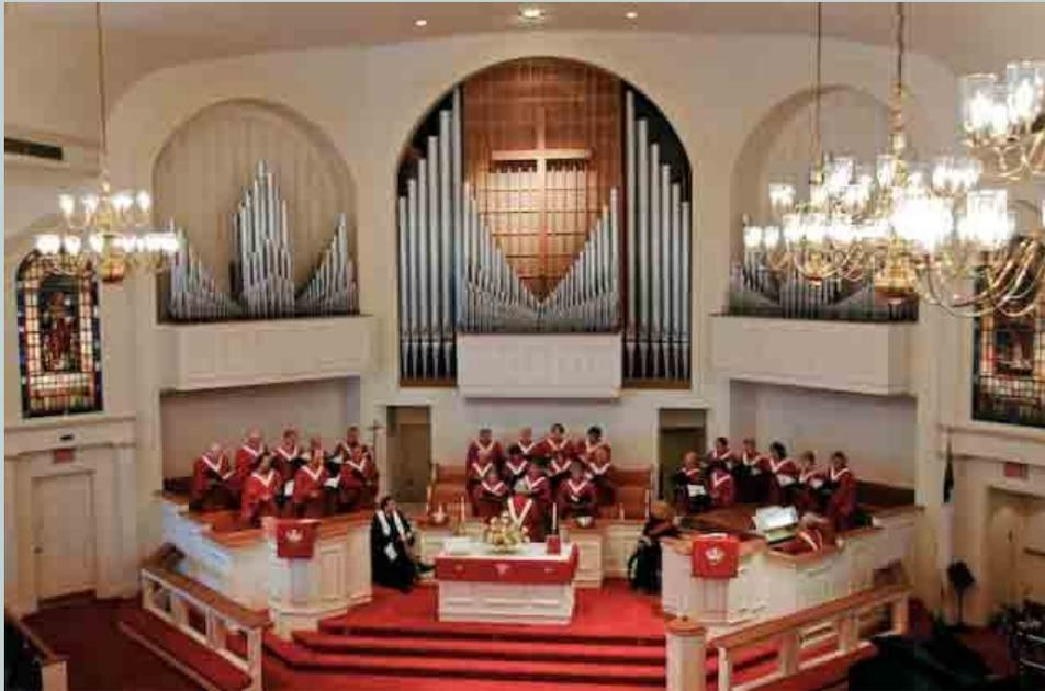
These curved surfaces cause "focusing" of sound creating many "hot" spots and unbalanced sound dispersion. Sound dispersion was designed to be kept away from these surfaces. The large chandeliers were also another area of concern due to the large glass globes which reflect sound in many different patterns. Care was taken in our design to make sure that sound
